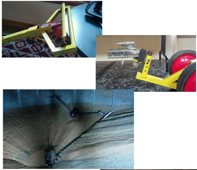
Engineering control must keep operator must at least 7' behind sweep auger at all times
