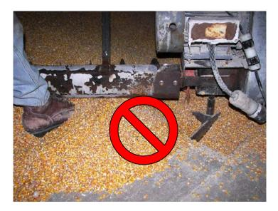
10. If maintenance/adjustments are necessary to the sweep auger, the auger must be unplugged, with the person making the adjustments maintaining the control of the plug, or locked-out in accordance with lock-out/tag-out procedures.
