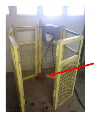
This is often referred to as a "whiskey barrel". Note the footoperated dead-man switch. 8. The auger is provided with a positive speed control mechanism or bin stop device that prevents the uncontrolled rotation around the bin. A hydraulically driven sweep auger is a positive speed control. The bin stop is for direct drive sweep augers.
