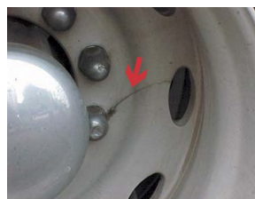
A crack extending between any two holes on a single wheel
