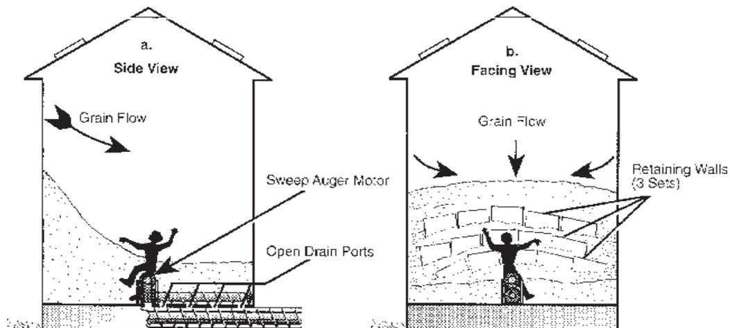
**Figure 1.** The initial grain flow trapped the victim's foot against the sweep auger motor, then proceeded to bury him above the waist (a). Three sets of retaining walls were established to prevent further grain flow around the victim and aid in grain removal with a vacuum conveyor (b).
