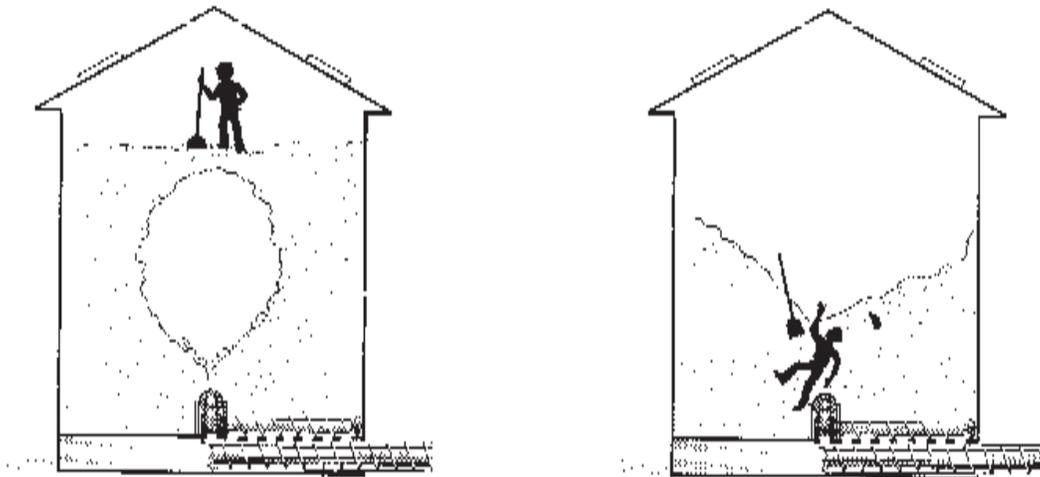
**Figure 3.** Grain can form a hard crust which appears to be firm enough to walk on. However, the crust can break and instantly bury an individual in the hollow cavity that formed underneath the bridge.
